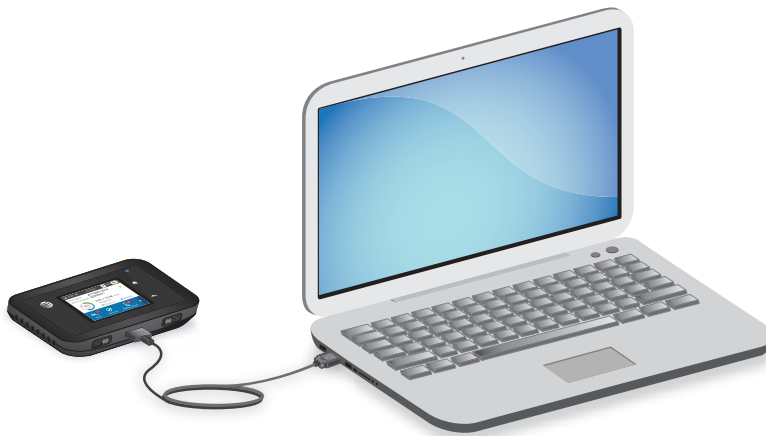
Figure 5. Use the USB cable to tether the mobile hotspot to your computer
